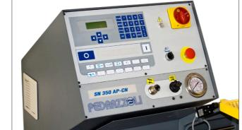
The control on the SN350 AP-CN is a PLC & N.C. specifically developed for automatic band sawing machines; it manages the machine by integrating the PLC functions for machine sequence with the N.C. functions for the management of the controlled axes which are the carriage advancement and how descent
