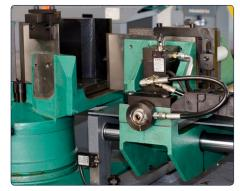
The vice on feeding carriage features a cylinder which permits to align the part with cutting vice so avoiding part scratching on main vice.
